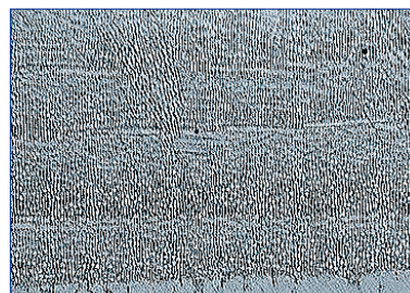
7 ■ Epitaxial growth on the directionally solidified superalloy MarM002.
