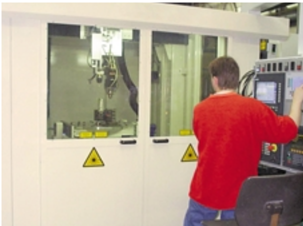
2 ■ The Sulzer Elbar laser center combines a welding and cladding technique for the repair of gas turbine components.
